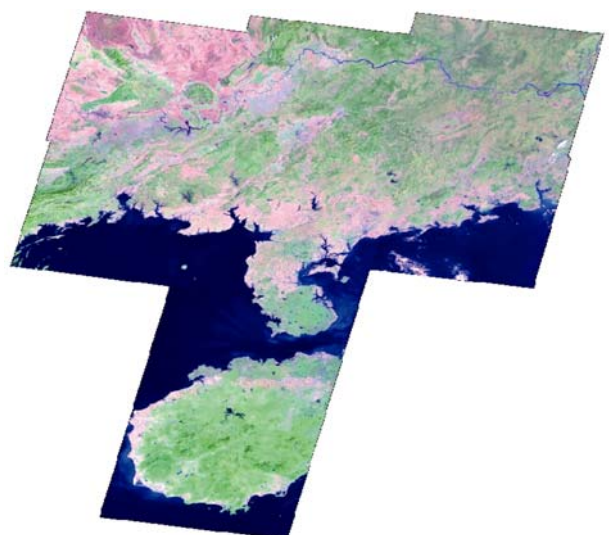
Fig. 6 The mosaic result using the method suggested in this paper and has few mosaic lines. The experimental results show that this method can calibrate differences of color and brightness in images of different time. Consequently, it can obtain satisfactory results on subsequent image classification and change detection.
